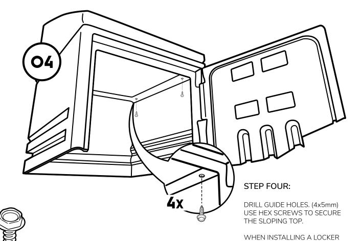
BANK, THE SLOPING TOP IS ONLY TO BE INSTALLED ON THE
